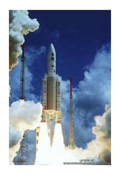
Exploded 37 seconds after takeoff - the reason was an overflow in a conversion of a 64 bit floating point number into a 16 bit integer.
