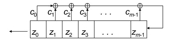
where the *i*<sup>th</sup> tap constant  $c_i = 1$ , if the switch connected, and  $c_i = 0$  if it is open. The contents of the register  $z_0$ ,  $z_1$ ,  $z_2$ ,  $z_3$ , ...,  $z_{m-1}$  are binary values. Given this state of the device the output is  $z_0$  and the new contents are  $z_1, z_2, z_3, \ldots, z_{m-1}, z_m$ , where  $z_m$  is computed using the recursion equation
