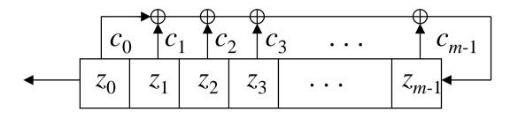
where the *i*<sup>th</sup> tap constant  $c_i = 1$ , if the switch connected, and  $c_i = 0$  if it is open. The contents of the register  $z_0, z_1, z_2, z_3, \ldots, z_{m-1}$  are binary values. Given this state of the device the output is  $z_0$  and the new contents are  $z_1, z_2, z_3, \ldots, z_{m-1}, z_m$ , where  $z_m$  is computed using the recursion equation
