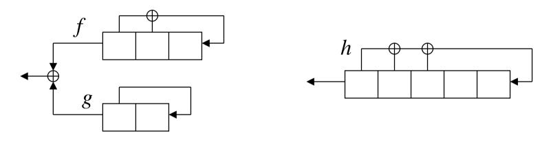
Further, if *f*-LFSR is initialized with 011, *g*-LFSR with 00, and the *h*-LFSR with 01110, then the two systems generate the same sequence: 011100101110010... Indeed, take the five first bits of any sequence generated by the *f* register and use them to initialize the *h* register. Then the *h* register generates the same sequence as *f* register.
