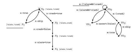
$$\begin{split} \Sigma_{system} &= \{ \texttt{s:true}, \ \texttt{s:skip}, \ \texttt{s:crash=true}, \ \texttt{s:crash=false}, \ \texttt{s:alarm=true} \} \\ \Sigma_{monitor} &= \{ \texttt{m:(!alarm&\&!crash)}, \ \texttt{m:(alarm&\&!crash)}, \ \texttt{m:assert(false)}, \\ &\quad \texttt{m:(crash)}, \ \texttt{m:true}, \ \texttt{m:skip} \} \end{split}$$
