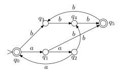
b) Language  $L = \{w \in \{a, b\}^* \mid w \text{ contains as many } a \text{ and } b \text{ letters modulo } 3\}$  is recognized by the following finite automaton:
