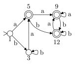
Now we notice that the automaton is already deterministic, so we may directly skip to the minimization phase. The minimization algorithm identify states 1 and 2 together, as well as states 6, 01, and 14. The resulting minimal automaton  $M_{r_1}$  is thus:
