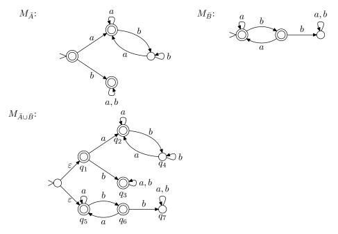
Before  $M_{\bar{A}\cup\bar{B}}$  can be complemented, it has to be determinised (the following automaton is minimal, details of minimization are left in appendix):
