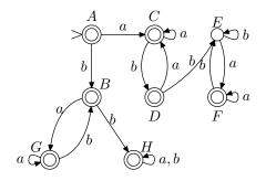
Now we want to find the minimal deterministic automaton that recognizes the same language. One algorithm is to define an equivalence relation  $\stackrel{0}{\equiv}$  on the set of states and refine it step-by-step until we reach the desired relation  $\equiv$ .
