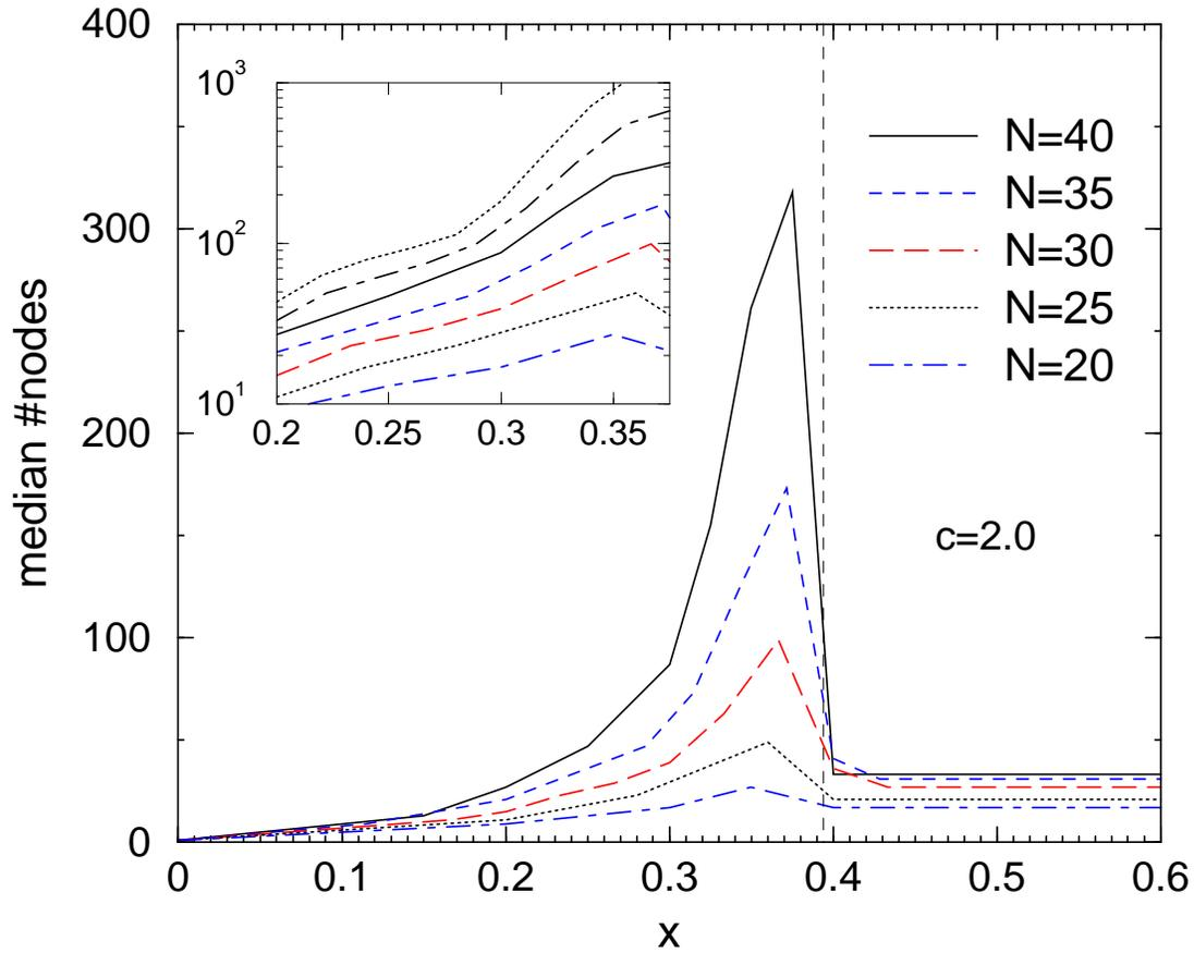
Figure 2: Time complexity of the vertex-cover algorithm = median number of nodes visited in the configuration.  $N = 20, 25, 30, 35, 40$ ,  $c = 2.0$ . Right part ( $x > 0.4$ ): Running times grows linearly. Inset: logarithmic scale (also  $N = 45, 50$ )  $\rightarrow$  time complexity grows exponentially with  $N$ .
