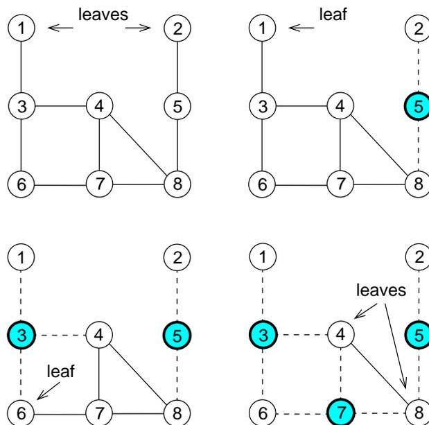
Figure 5: Example of the leaf-removal algorithm. Upper left: initial graph, vertices 1 and 2 are leaves. Upper right: graph after the first iteration, vertex 5 has been covered (shown in bold) and the incident edges removed (shown with dashed line style). Bottom: graph after second and third iteration.
