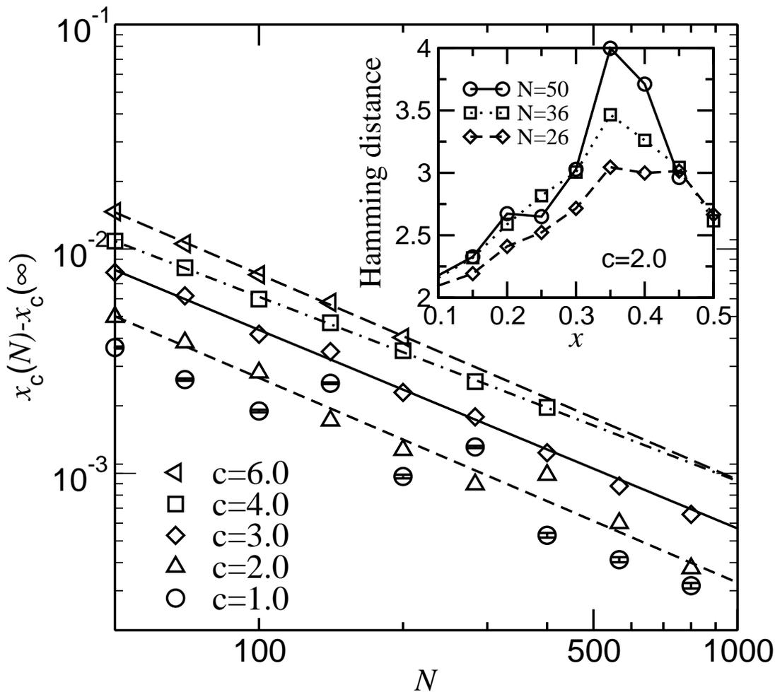
Figure 3: Finite-size scaling behavior of the critical cover size. The location of the transition point  $x_c(N)$  as a function of graph size  $N$  for different average degree  $c$ . Inset: scaling of the correlation volume as a function of  $x$  for different sizes. Error bars are, at most, of the order of the symbol size.
