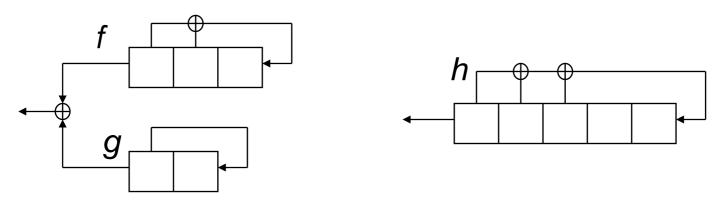
Further, if *f*-LFSR is initialized with 011, *g*-LFSR with 00, and the *h*-LFSR with 01110, then the two systems generate the same sequence: 011100101110010... Indeed, take the five first bits of any sequence generated by the *f* register and use them to initialize the *h* register. Then the *h* register generates the same sequence as *f* register.
