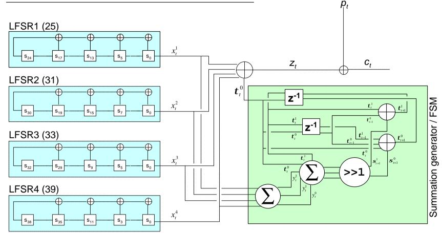
(4,4)-combiner: four LFSRs and memory bits  $(t_{t-1}^0, t_{t-1}^1, t_t^0, t_t^1)$
