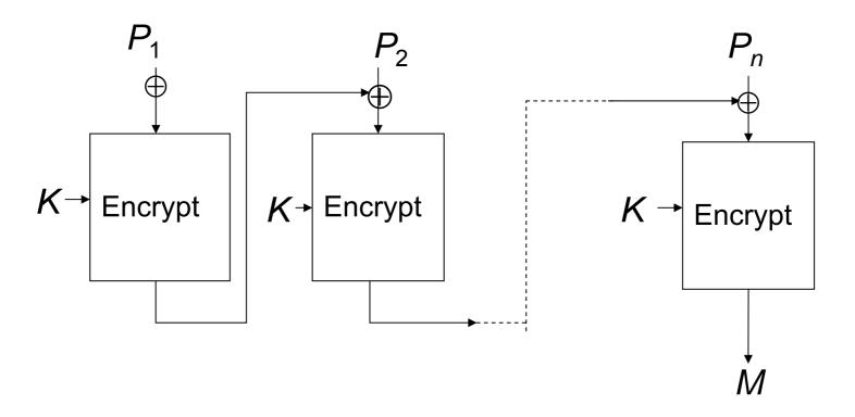
CBC encryption with fixed IV = 00...0. The last ciphertext block (possibly truncated) is taken as the MAC.
