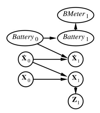
Both position (evidence variables  $\mathbf{Z}_t$ ) and the battery charge level (evidence variable  $BMeter_t$ ) are measured.
