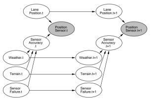
➤ The model for the variable SensorFailure determines that the sensor usually stays broken once it gets broken.
