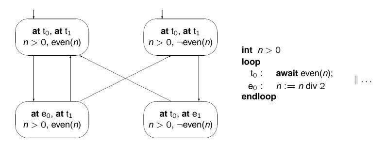
No computation of "concrete" system cycles between left-hand nodes
