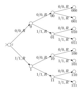
If the machine ends in the state 011, then the input symbol is  $a_3$  since  $011_2 = 3_{10}$ . The symbol that is written to the tape is similarly done using k different transitions. Finally, the tape head is moved k steps to the correct direction.
