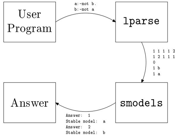
Figure 1.1: The way of a logic program
