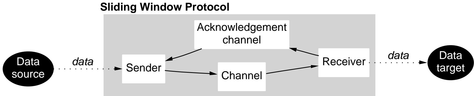
We have constructed a model of the protocol in the MARIA modelling language (roughly 200 lines of text). In this variation, two kind of messages are sent until a third kind of message ends the transmission. The sender and the receiver have a buffer for 1 message. The reachability graph contains 264 states and 582 arcs. If the transmission was continuous, the initial state would be reachable from each reachable state, and the reachability graph would thus have one *strongly connected component*.
