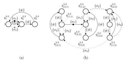
Fig. 8.1: Examples of automata used in the proof of Proposition 8.2.1. (a) The automaton  $\mathcal{A}_{3,3}$ . (b) Automaton obtained from  $\mathcal{A}_{3,3}$  via degeneralization
