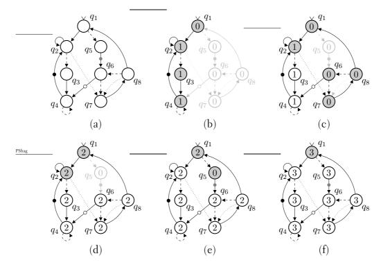
Fig. 8.3: Example on running the emptiness checking algorithm on an automaton. (a) An automaton with three acceptance conditions and a nonempty language; (b)–(f) State of the algorithm when the top-level search is about to backtrack from the states  $q_4$ ,  $q_6$ ,  $q_2$ ,  $q_5$  and  $q_1$ , respectively
