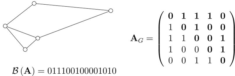
Figure 6.1: A graph  $G$  of order five, an adjacency matrix  $\mathbf{A} = \mathbf{A}_G$  with the entries that form the bit string in boldface, and the corresponding bit-string representation  $\mathcal{B}(\mathbf{A})$ .
