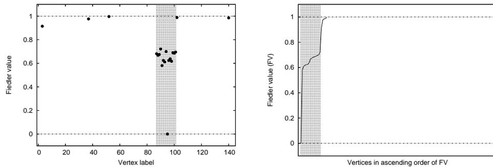
Figure 4.8: Components of a Fiedler clustering vector sorted by index (left) and in ascending order (right). The vertical lines represent the cluster selection of the Cheeger-ratio local optimization method based on the Fiedler values.
