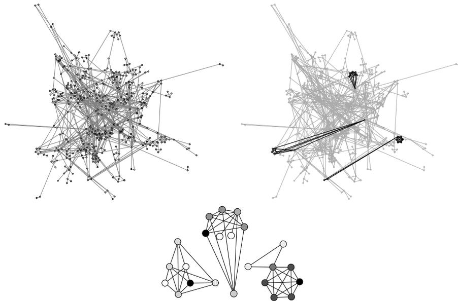
Figure 4.9: Local Fiedler clusters in a 503-vertex collaboration graph; on the bottom, a closeup view of the three clusters with distant and overlapping vertices rearranged to allow a better view of the structure of the induced subgraphs.
