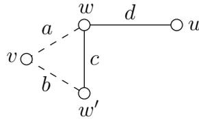
Figure 5.8: A small example graph where vertex  $v$  needs to choose whether to link to  $w$  or  $w'$  (the dashed edges) to form a spanning tree used to route communications. Edge weights ( $a, b, c, d$ ) are shown next to the arcs; the length of the edges in the drawing is does not reflect the weights. We set  $a > b$ .
