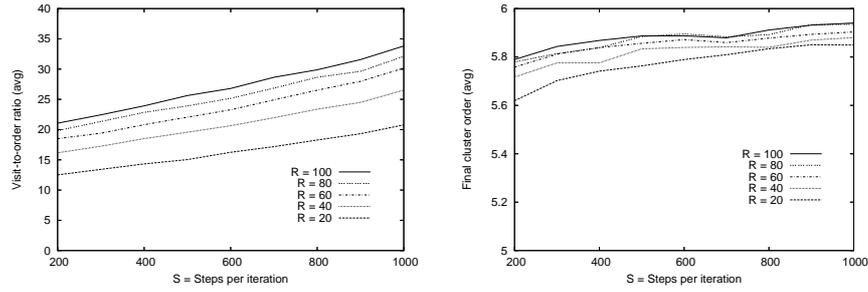
Figure 4.5: On the left, the ratio of the number of vertices visited (i.e., the visit count for an  $R/S$ -pair) to that of the number of vertices selected in the final cluster (i.e., the cluster order) averaged over 100 vertices selected uniformly at random and repeated 50 times per vertex. On the right, the average final cluster orders of the same experiment set.
