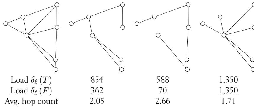
Figure 5.6: A small graph (on the left) with three possible spanning trees: a random one, a line, and a star topology. Below the pictures are the values for two possible global load measures (using the vertex-betweenness) and the average hop count (calculating the hop-distance for each pair of distinct vertices once).
