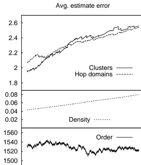
Figure 4.17: The evolution of the average and standard deviation of the estimate error for a caveman graph during 1,000 modification operations. The density and order of the graph after each modification step are also plotted to reveal the type of modifications that occurred; the start order is 1,533 and the initial size 50,597.
