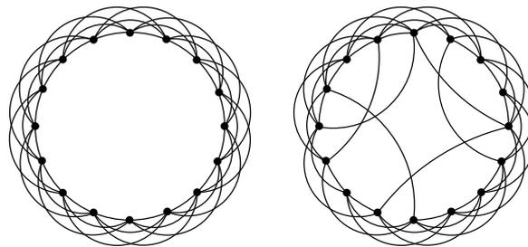
Figure 2.1: On the left, the initial lattice graph of Watts and Strogatz with  $n = 16$  and  $k = 3$ ; on the right, a rewired version with small  $p_e$  (adapted from [314]).
