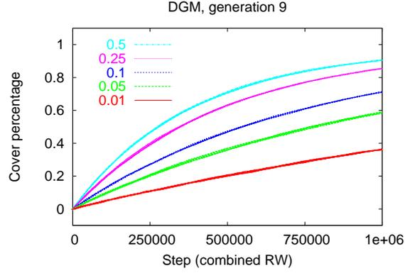
Figure 3.8: The behavior of the combined random walk on a ninth generation graph for different values of  $\epsilon$ . Increase in coverage is only measured at sampling steps, i.e., the vertex visits of the mixing side of the construction are not counted in the coverage but are present in the step count.
