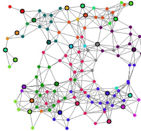
Figure 4.12: Each cluster has its own color; the nodes have been added one by one, with existing nodes updating their clusters after the newcomer selects a cluster. Cluster heads are drawn with a black border. In these examples, all nodes have a fixed communication range and they do not move.
