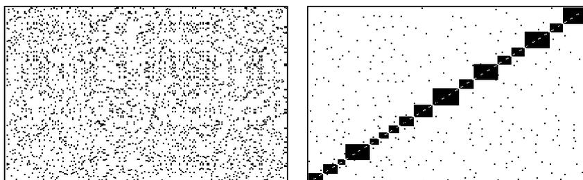
Figure 4.4: The adjacency matrix of a caveman graph with 210 vertices and 1,505 edges; the left one uses random vertex order, reflecting little structure, whereas the one on the right is sorted by the clusters found by locally optimizing Equation 4.30 — the sorted matrix clearly reveals the cave-based structure.
