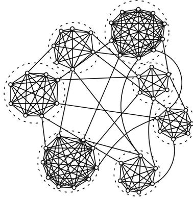
Figure 4.3: An example caveman graph with 55 vertices and 217 edges; each cave (encompassed by a dotted line) is correctly identified as a cluster by the local optimization of Equation 4.30.
