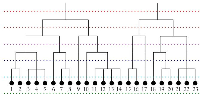
Figure 4.1: An example dendrogram that groups 23 elements into clusters at four intermediate levels, the root cluster containing the entire dataset and the leaf clusters each containing one data point. Any level of the dendrogram, indicated by dotted lines in the picture, can be interpreted as a clustering, grouping together as a cluster those elements that remain in the same branch of the dendrogram tree above the line.
