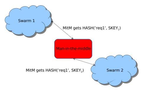
Fig. 5. Torrent fingerprint by man-in-the-middle in two swarms.
